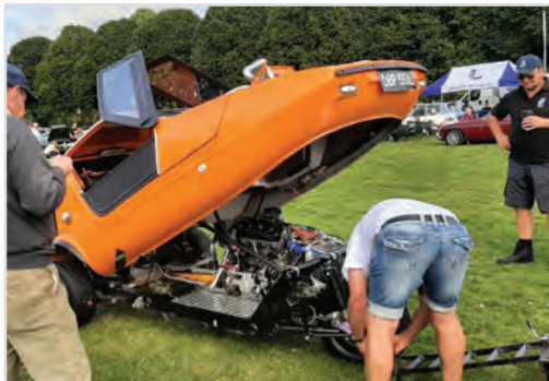
Bug has an interesting modification with a lift up body to improve engine access
